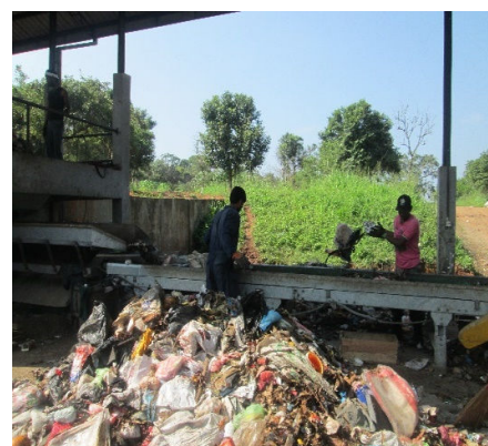
Figure 6: Manual waste segregation by conveyor belts (Anuradhapura)
