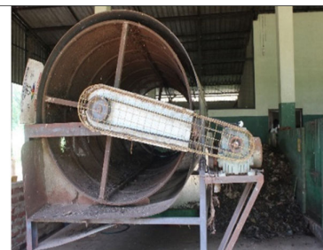
Garbage separation equipment
